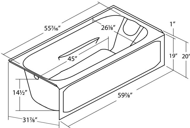
Left-hand drain shown—reverse layout for right-hand drain.
