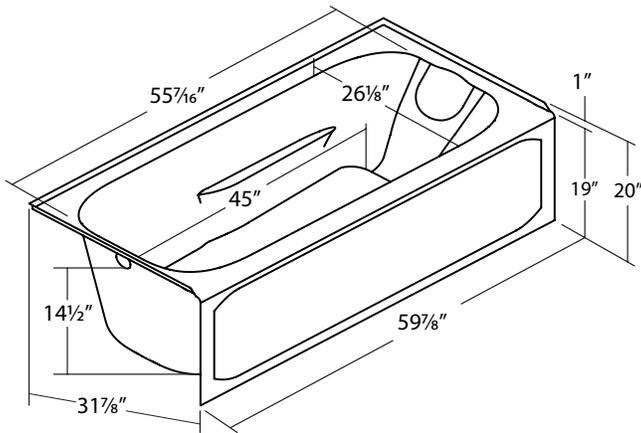
Left-hand drain shown—reverse layout for right-hand drain.
